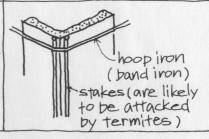
this reinforcement prevents the spreading of walls and increases the strength of the building
