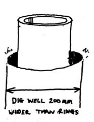
The top of the pit must be secure. Timber shuttering must be made if the soil is loose or sandy.
