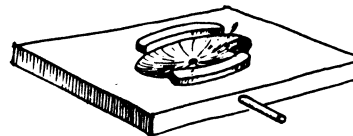
Vietnamese proposal for a squatting plate where the removable drain closes one vault and leaves a drop hole for the other vault. Now the urine tank can be placed inside the toilet base.
