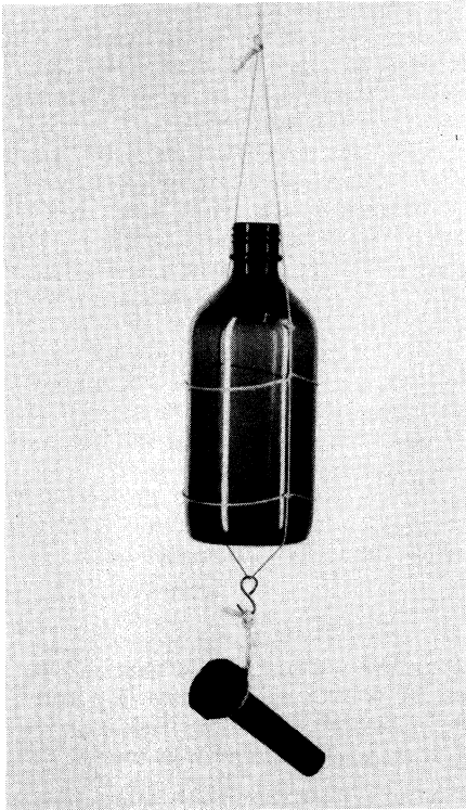
Fig. A1. A weighted bottle for sampling from wells.
