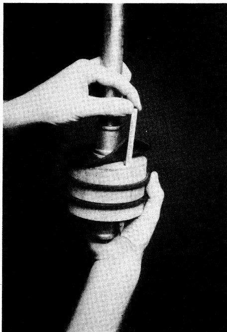
Fig. 15. A surge plunger for a 100 mm diameter tube well. The holes run right through the plunger, except for the top flap.
