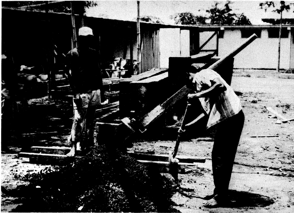
Figure 3 Tek-Block press in use
