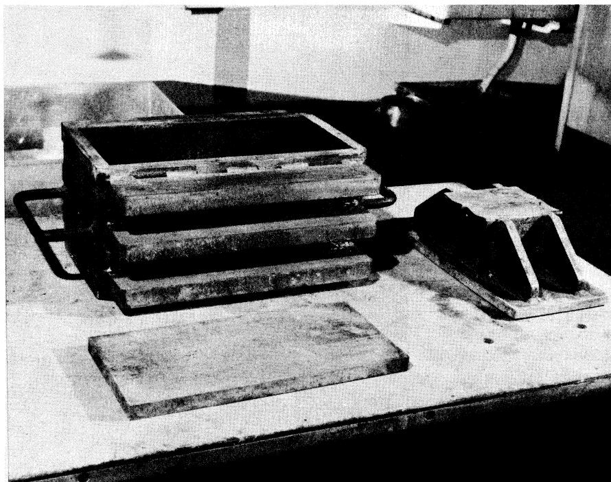
Figure 5 Reinforced mould for making blocks at high compaction pressures
