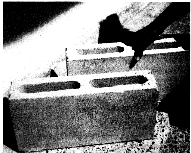
Figure 21 Blocks made from rha cement (front) and OPC (back) during weathering test in Guyana
