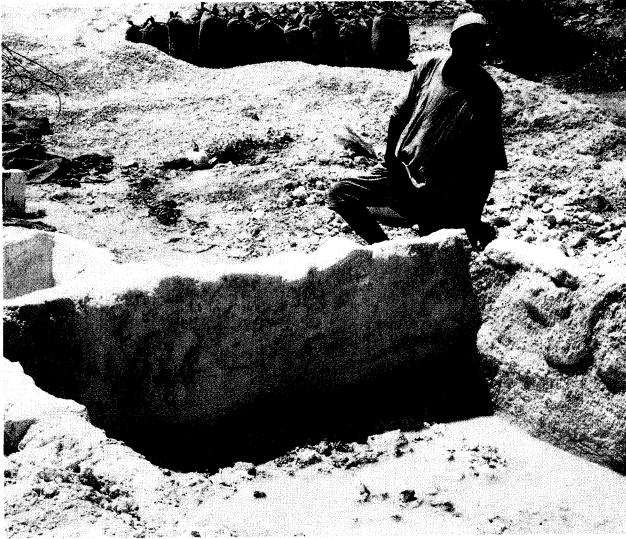
Figure 4 Slaking quicklime in Sudan
