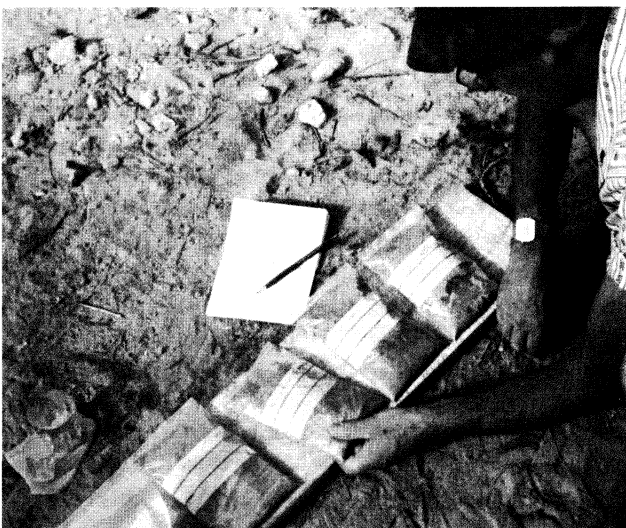
Figure 15 Experiment with fish glue as plaster retarder in Cape Verde
