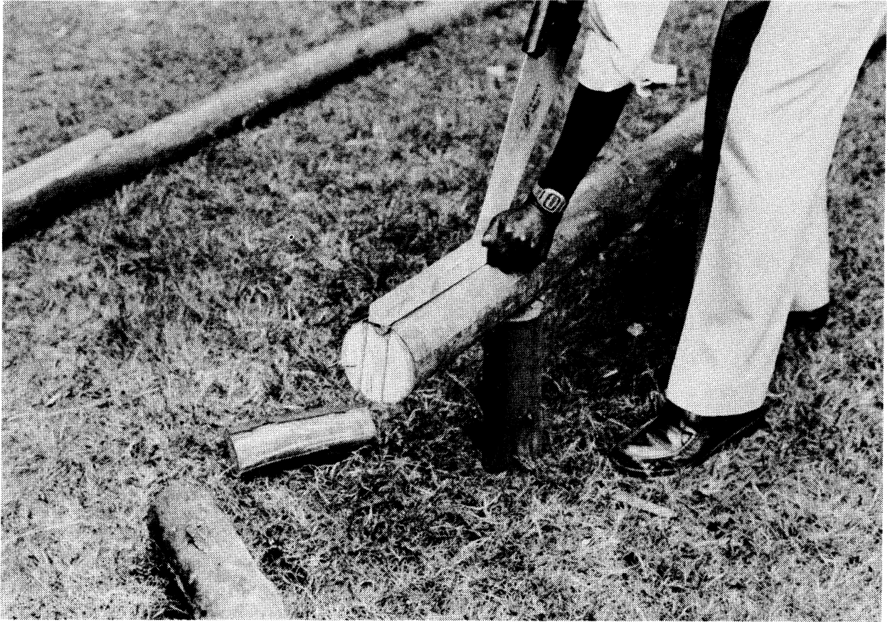
Plate 9 Use of a guide for making parallel saw cuts
