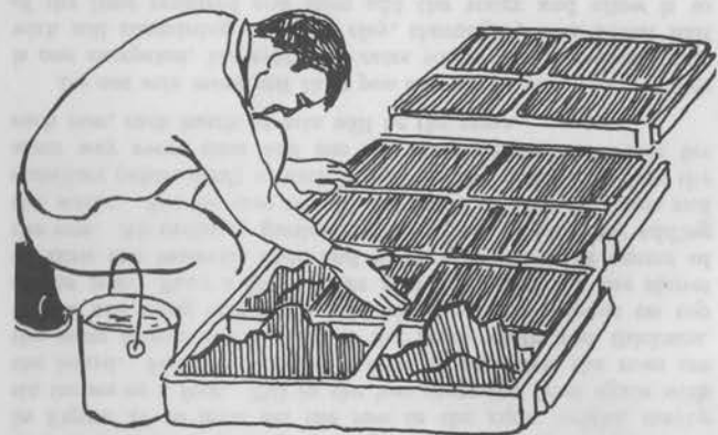
Figure 40. Kneading and leveling the blocks.
